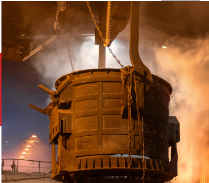
Argon stirring at Ladle Furnace
